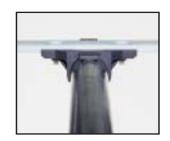
**BOLT-ON VERSION -** When roller removal is desired, the **EZ Roller Retrofit Bolt-On Component** is recommended. Sturdy 5 foot sections are pre-assembled to save labor, and bolt into existing roller 7/16" (11 mm) hex holes (only eight bolts per section required). A chevron wearstrip pattern increases belt life.
